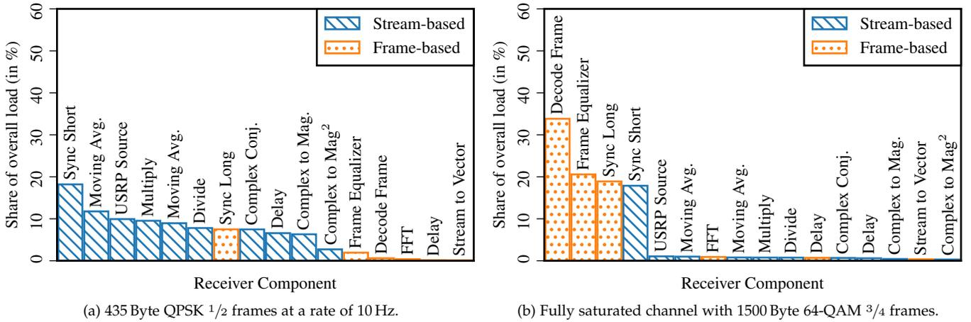
Figure 6. Computational demands of individual signal processing blocks.
