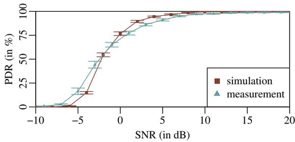
Figure 7. Simulated packet delivery ratio at different SNR levels.
