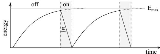
Figure 3. Qualitative overview of the charging and discharging process of the capacitor and the duty cycle of the transceiver.
