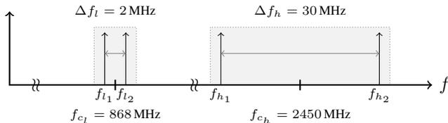
Figure 2. Signal design with multiple coherent carriers.
