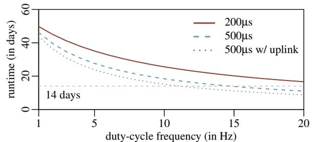
Figure 6. System runtime dependent on duty cycle and burst configuration.
