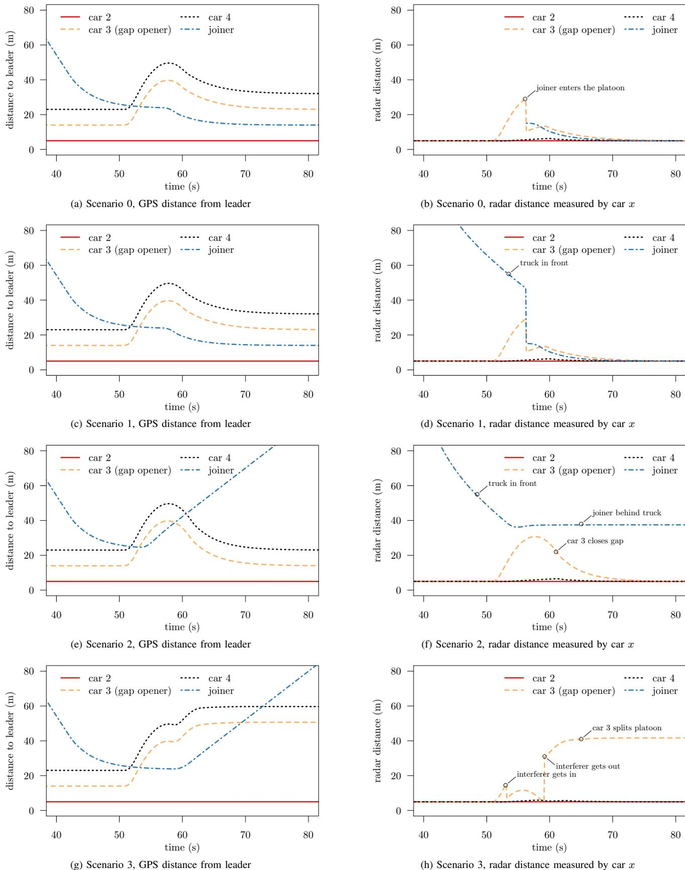
Figure 5. Vehicles dynamics for the different scenarios: left plots show the GPS distance to the leader; right plots show the measured radar distance.
